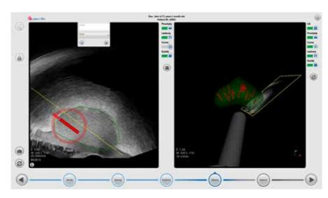
Fusion Bx software guides users through the fusion biopsy procedure in 5 simple steps, while advanced 3D visualization allows fast tracking and targeting
